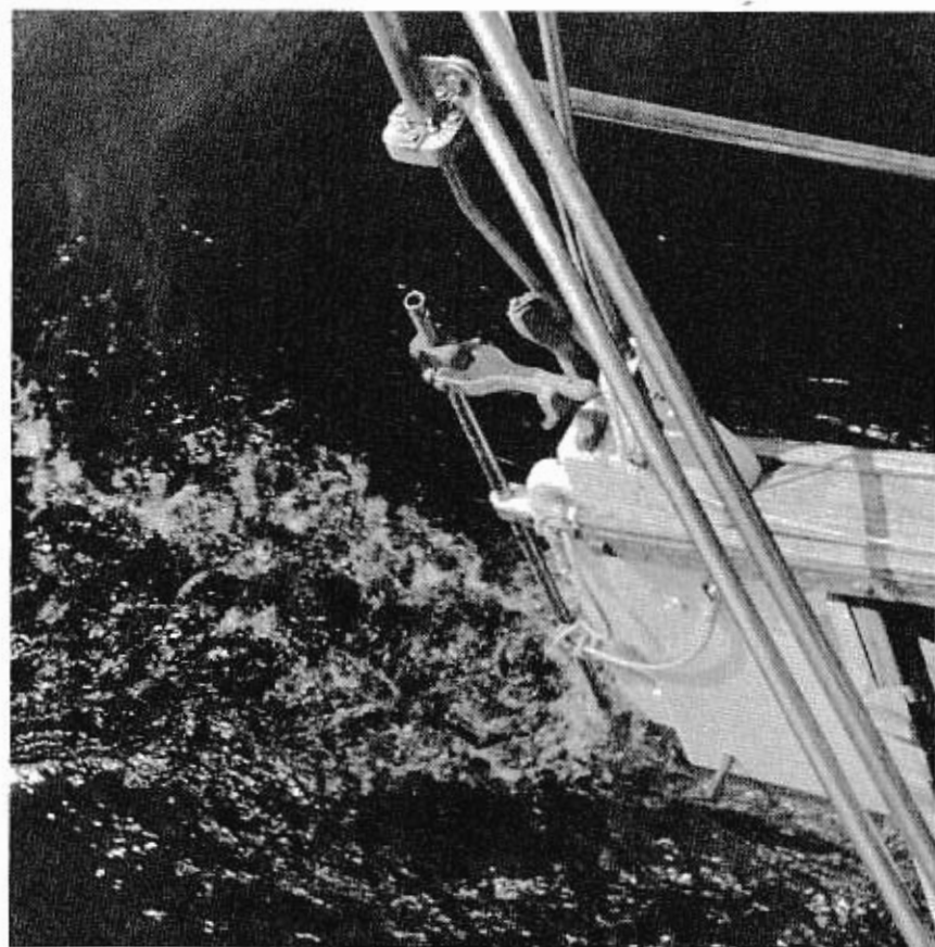
Aleutka's feedback linkage.
