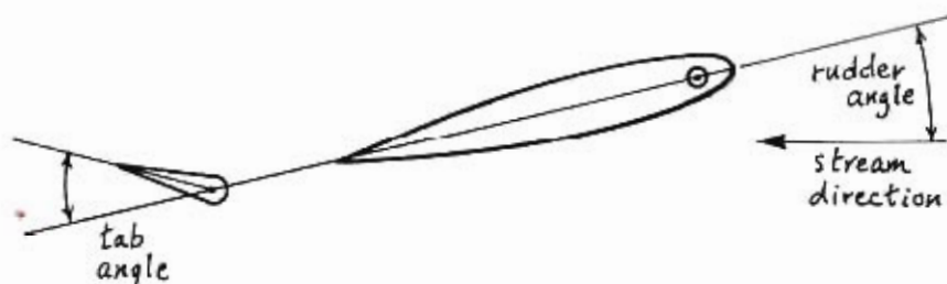
5-36. Tab angle is measured from the plane of the rudder.
