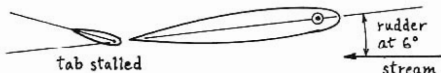
5-38. Example of tab with volume only half the rudder self-volume.
