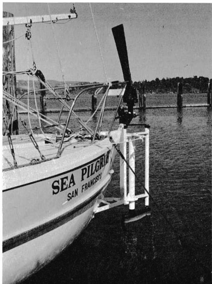
The Polaris gear uses a horizontal-axis vane, feedback linkage, and a servo tab operating a balanced auxiliary rudder — a very powerful combination. Photo courtesy of James F. Ogg & Associates.
