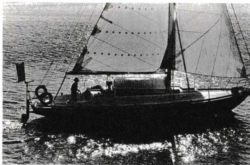
Hal and Margaret Roth's Spencer-35 Whisper with her new Riebandt auxiliary rudder/servo tab gear and a wedge-section vertical-axis vane. She was fitted with a Hasler servo pendulum vane gear for her voyage from San Francisco via many islands to Japan and back.
